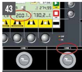
43 SHARK 350 CNC HS 4.0 / SHARK 350 NC HS 5.0 Kit vitesse ruban 15+200 m/min
