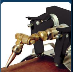
Allows the torch tip to be adjusted for any angle from a square cut (no bevel) to a bevel angle up to 90 degrees while also allowing torch lead or lag angle adjustment.
