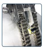
MagSquare magnets are now standard with all double chain clamps to make setup simple and easy.
